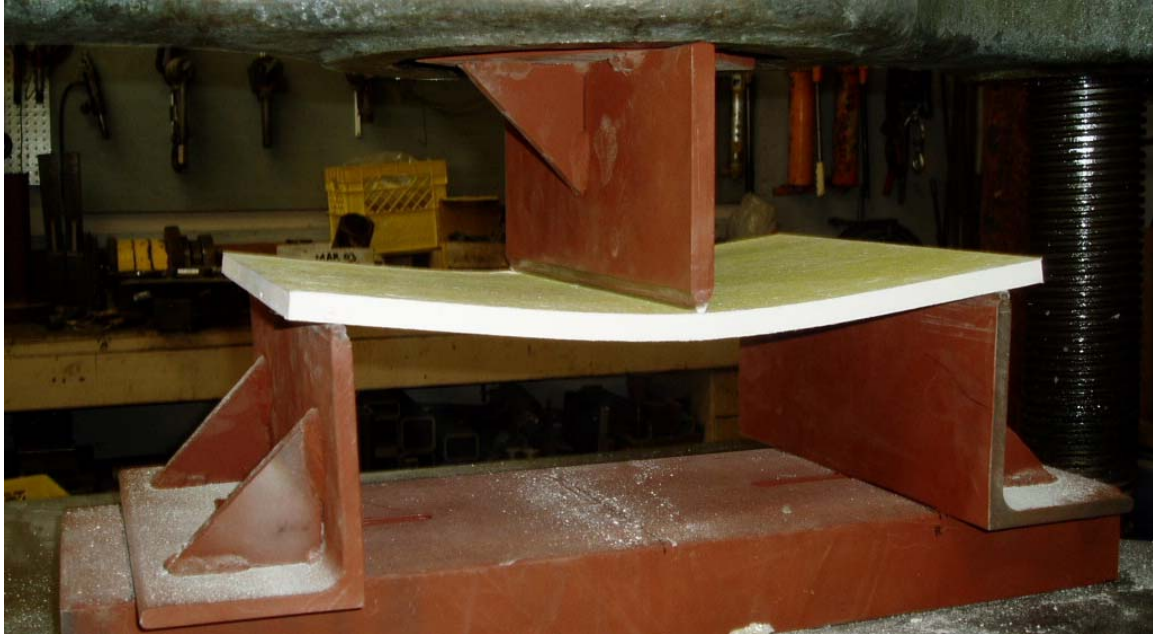
FIGURE 1B. TESTING APPARATUS FOR FLEXURAL STRENGTH
