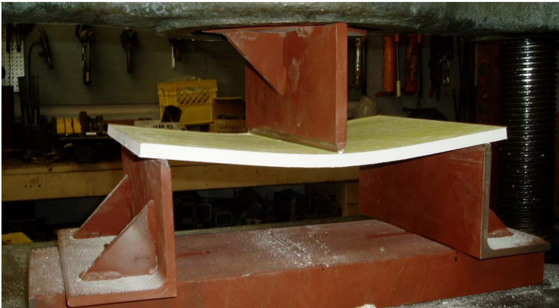
FIGURE 2. TESTING APPARATUS FOR FLEXURAL STRENGTH
