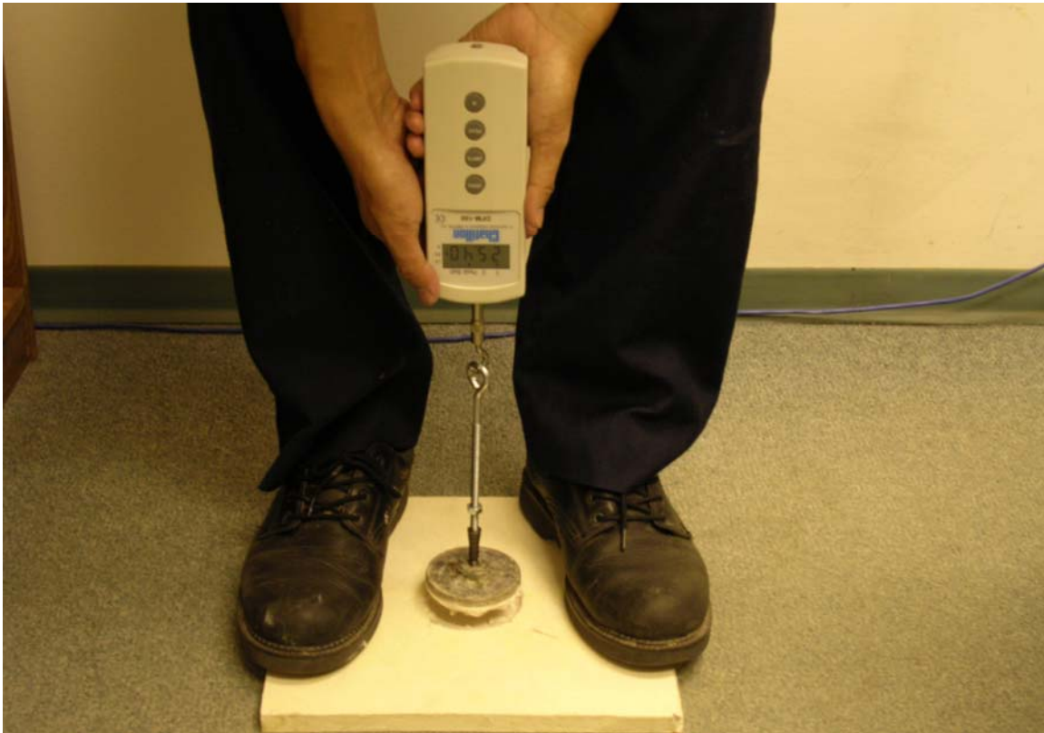
FIGURE 3. TESTING APPARATUS FOR FACER DELAMINATION
